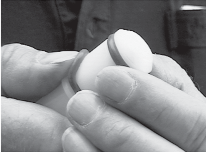
Figure 23. Removing "O" Ring
