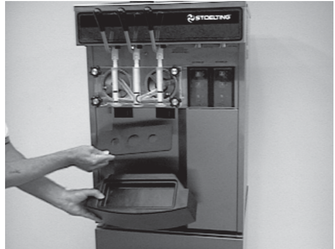
Figure 5. Installing Tray and Insert
