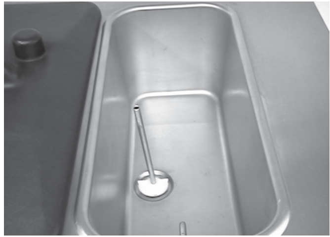
Figure 26. Install Mix Inlet Regulators
