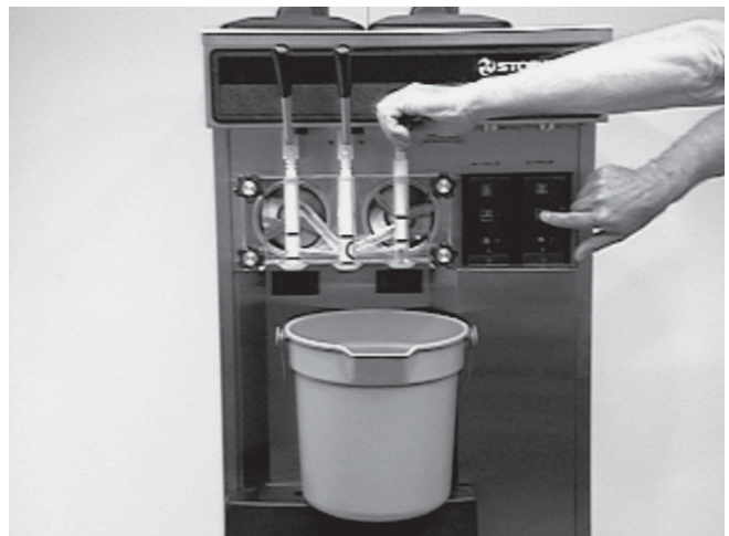
Figure 14. Spigot Opened and Solution Draining
